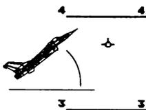
Represents your plane's angle of climb. When positive numbers (0 through 9) are showing, the plane is in an upward climb. Negative numbers (-0 through -9) signify a dive. Each number represents an increment of ten degrees, from 0° to 90° in either direction. The ladder displayed here shows the F-16 in a 38 degree climb. (Negative numbers also shown by dotted line.)
